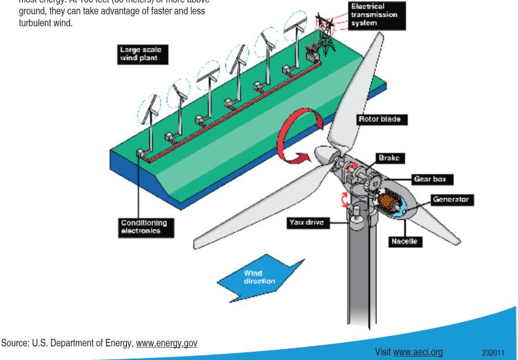
**Rotor:** The blades and the hub together are called the rotor. Most turbines have either two or three blades. Wind blowing over the blades causes the blades to "lift" and rotate. Blades are turned, or pitched, out of the wind to keep the rotor from turning in winds that are too high or too low to produce electricity.
